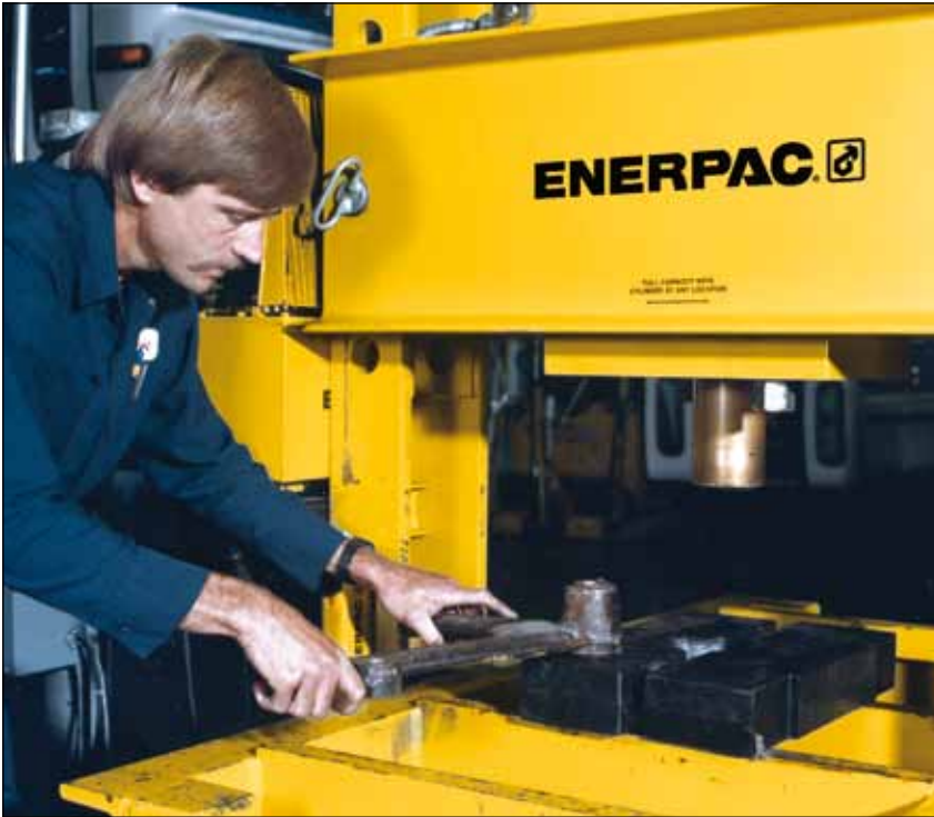
▲ A BPR-20075 Roll-Frame Press is used to remove a large shaft from this pillow-block assembly. The Roll Frame design allows this heavy part to be safely loaded with an overhead crane.
