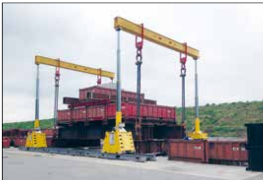
◀ SL-400 Gantry during load testing.
