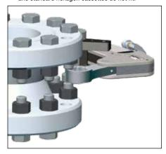
▼ The WCR-wrench must be removed and repositioned after each wrench cycle by operating the pump in the retract direction. The tool contains no spring return.
