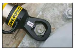
Heavily corroded and weathered nuts are quickly split and removed using a NS-Series Nut Splitter.
