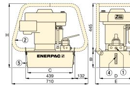
User adjustable relief valve on all manual valves. 3/8" NPTF on A and B ports; 1/4" NPTF on auxiliary ports. (2) Roll Bar
