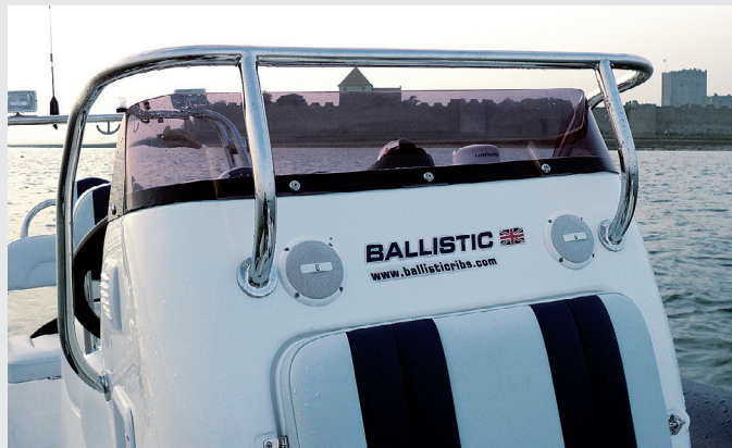
ABOVE: Well finished stainless steel grab rail to steering console.
