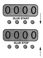
If you need to revert to normal running at any time just press the two left hand switches together (as in zeroing glue line settings) and then enter start and stop positions in the normal way. Remember that you will need to change the settings in Prg Code back to normal as well!
