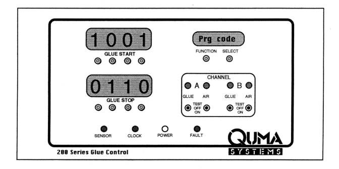
Using the FUNCTION switch to scroll down to Prg Code allows the plant engineer to access the calibration section of the controller.
