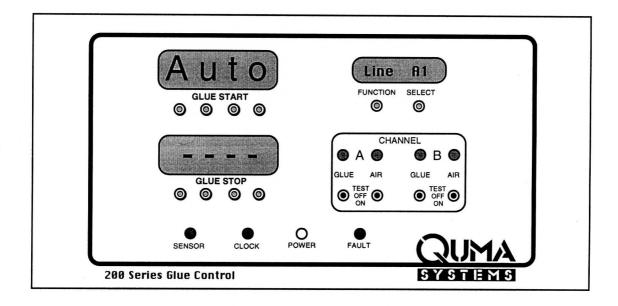
If the sensor is mounted in line with the glue application head it is possible to glue tabs automatically. Press the two end switches together and 'Auto' will appear in the GLUE START window.
