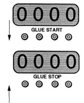
Please remember that you do not have to clear settings in all 8 glue positions. An all ZERO entry in any position will stop the controller from continuing to the next position.
