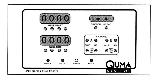
The control has now changed to glue line setting function and "Line A!" will have appeared in the function window. The way that the position of the glue lines is entered is as follows:
