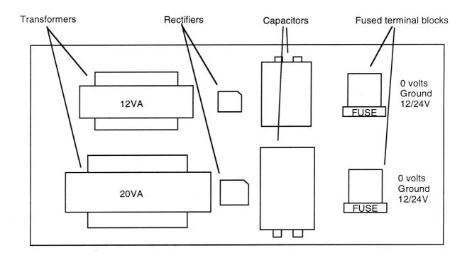
In this twin power supply the 12VA transformer supplies power to the MAC 200 pcb only. The 20VA transformer supplies the input / output devices.
