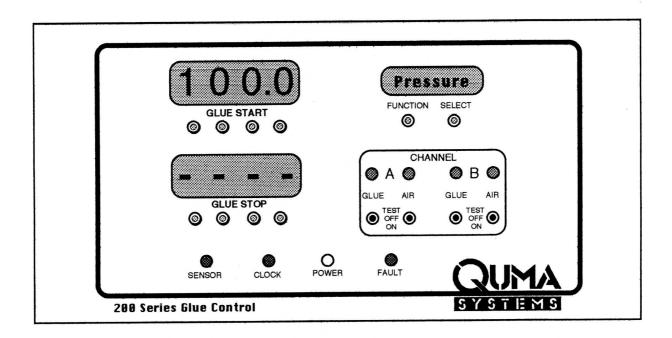
If the system is being run with glue / speed compensation then pressing the FUNCTION switch once more will display "Pressure" in the function window.
