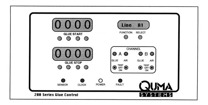
To save time when entering glue line positions it is possible to zero the number displayed in the GLUE START and STOP windows.
