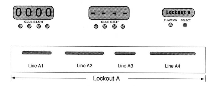
If using channel B then the "Lockout B" is selected by depressing the FUNCTION switch again after "Lockout A" and the dimension set in the same way.
