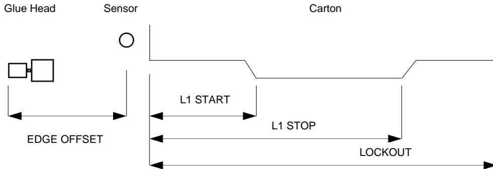
This shows an alternative installation which will allow the use of Normal or Automatic gluing because the sensor is in line with the glue head. This shows the measurements required for NORMAL gluing. Please note the change of reference point!
