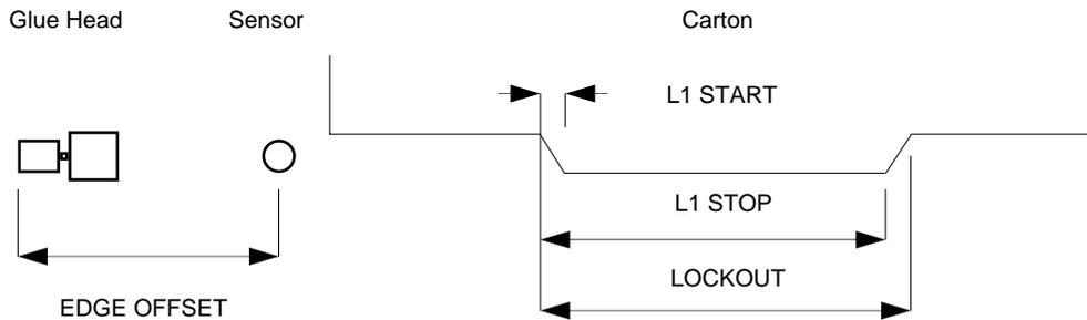
In this operation when AUTOMATIC is selected the GLUE RADIUS setting fixes the distance that the glue starts and stops from each end of the glue tab whatever the carton length. Adjust EDGE OFFSET to centralise the glue pattern on the glue tab.
