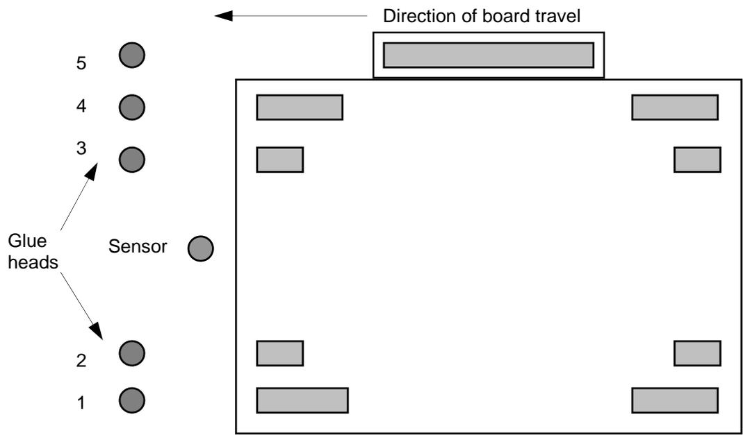
In the above example the system is driven by a 3 channel controller with five glue heads.
