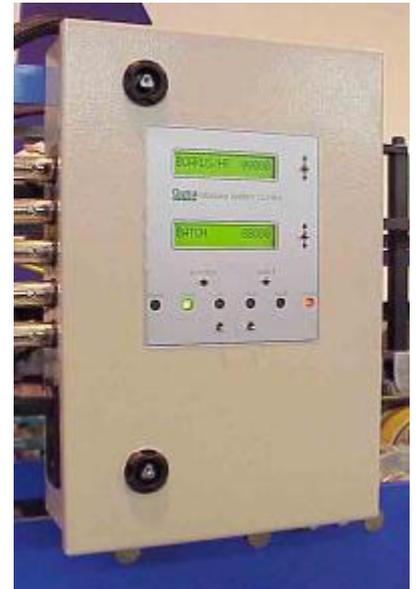
The controller is a sophisticated counter system. It receives pulses from an encoder running at belt speed or from the internal pulse generator on fixed speed machines. The infra-red optical sensor picks up the leading edge of the box and initiates a count sequence and a series of calculations to determine precise start and stop positions for the glue application.
