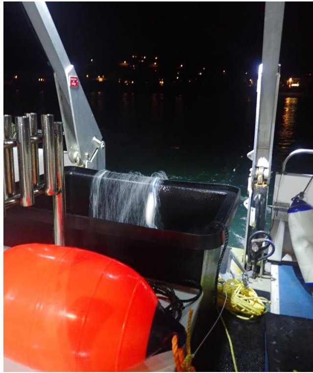
Figure 5: Net being deployed through the A-frame of Tiger on the 18 th March 2019
