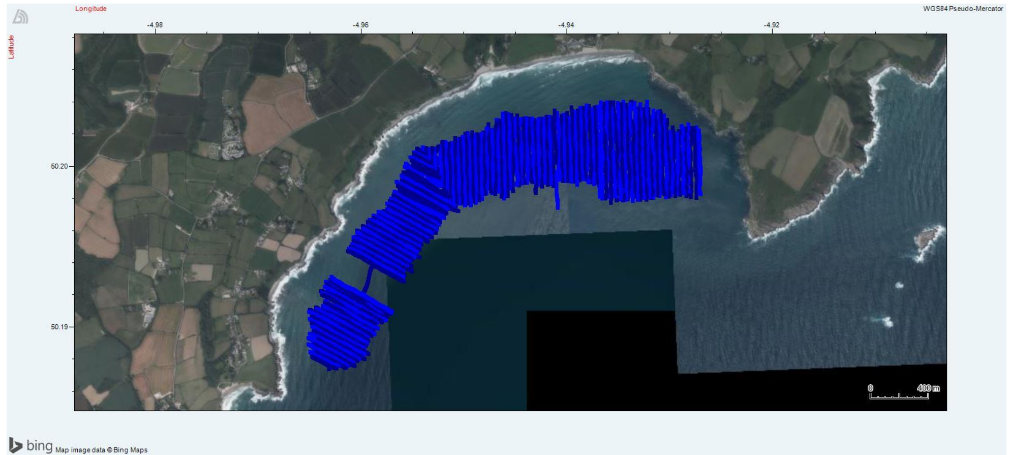
Figure 1: Acoustic survey lines completed within Gerrans Bay using an MX Echosounder by Cornwall IFCA 2022.
