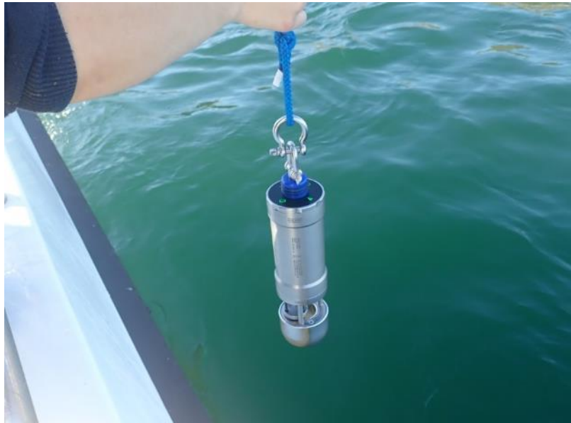
Annex Figure D: Valeport Swift Sound Velocity Profiler deployed from R/V Tiger Lily VI
