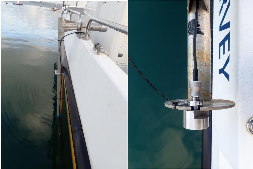
Annex Figure B: Pole mount and MX Acoustic Echosounder onboard R/V Tiger Lily VI
