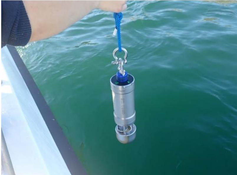
Annex Figure C: Valeport Swift Sound Velocity Profiler deployed from R/V Tiger Lily VI
