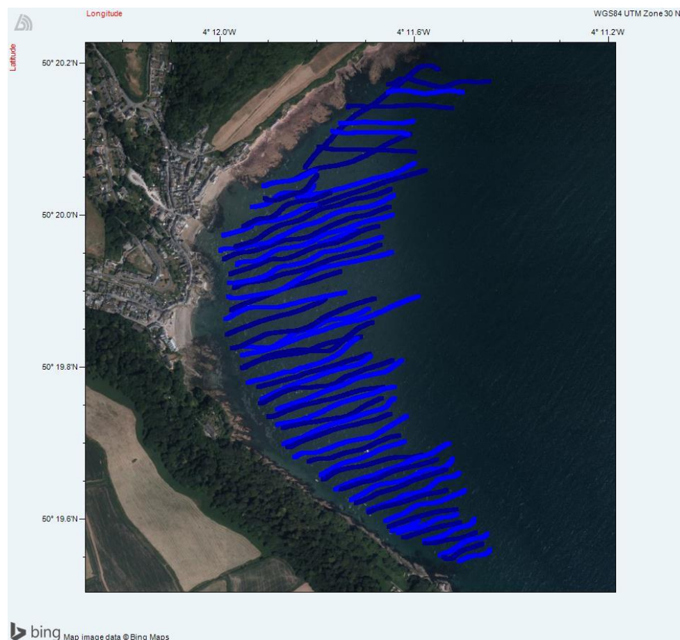
Figure 1: Acoustic survey lines completed at Cawsand using an MX Echosounder by Cornwall IFCA 2021.
