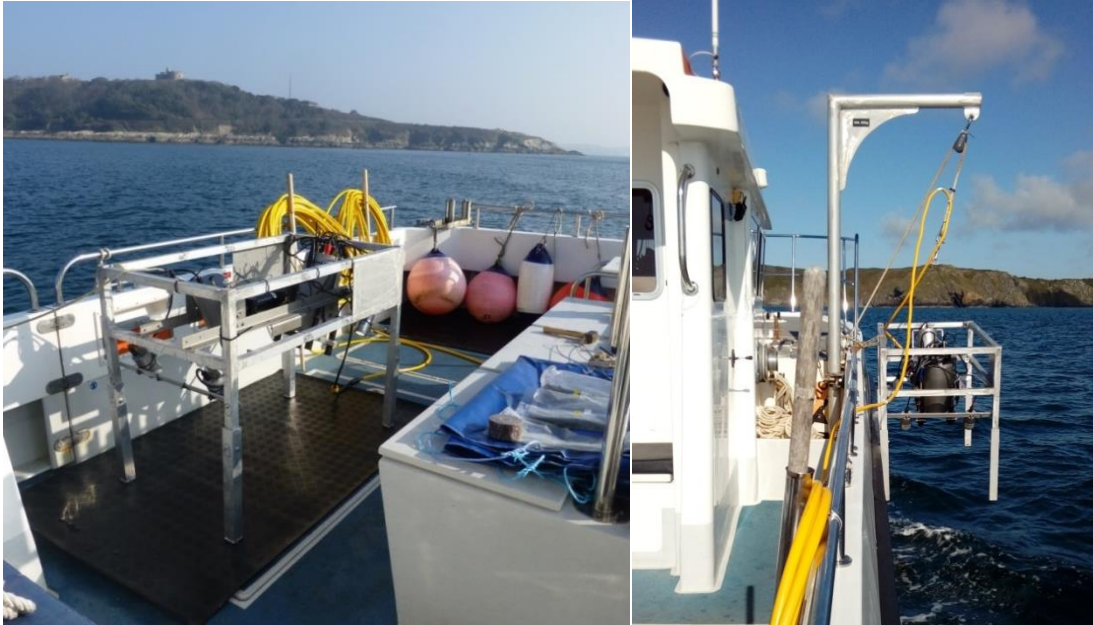
Figure 4: SeaSpyder drop camera housed in a purpose built frame on the aft deck and in the deployment position onboard R/V Tiger Lily VI.
