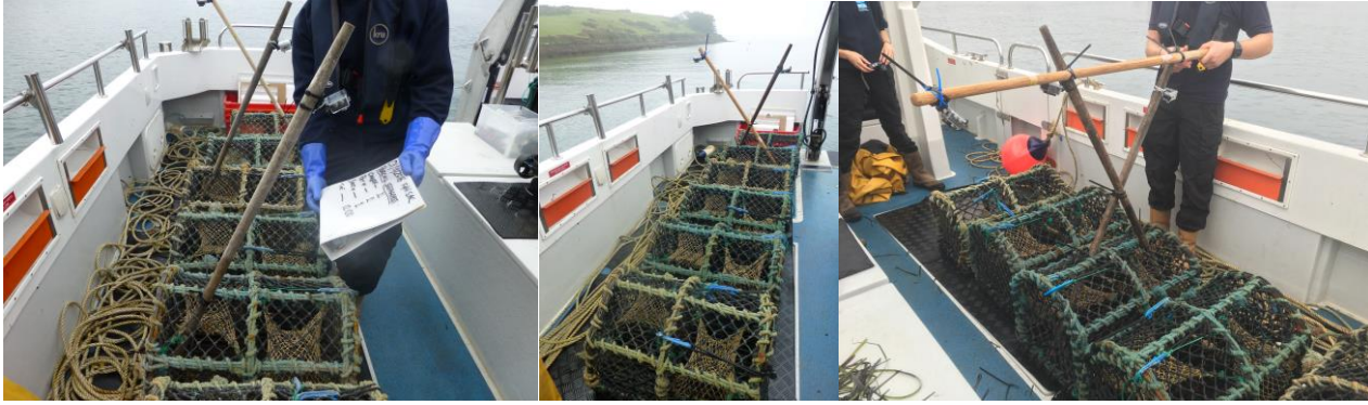
Figure 3: The six pots set up on the starboard side of R/V Tiger Lily VI with the survey poles and camera housing attached. The positions from left to right are position 1, position 2 and position 3 which are described above
