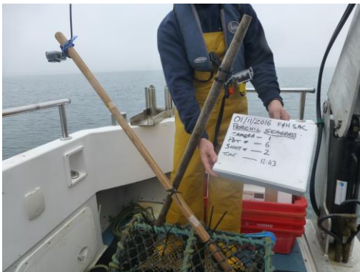
Figure 4: An example of the deck slate in use and the set up of the poles and cameras used for the survey
