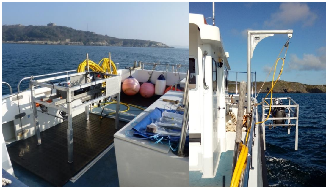
Figure 5: SeaSpyder drop camera housed in a purpose built frame on the aft deck and in the deployment position onboard R/V Tiger Lily VI.
