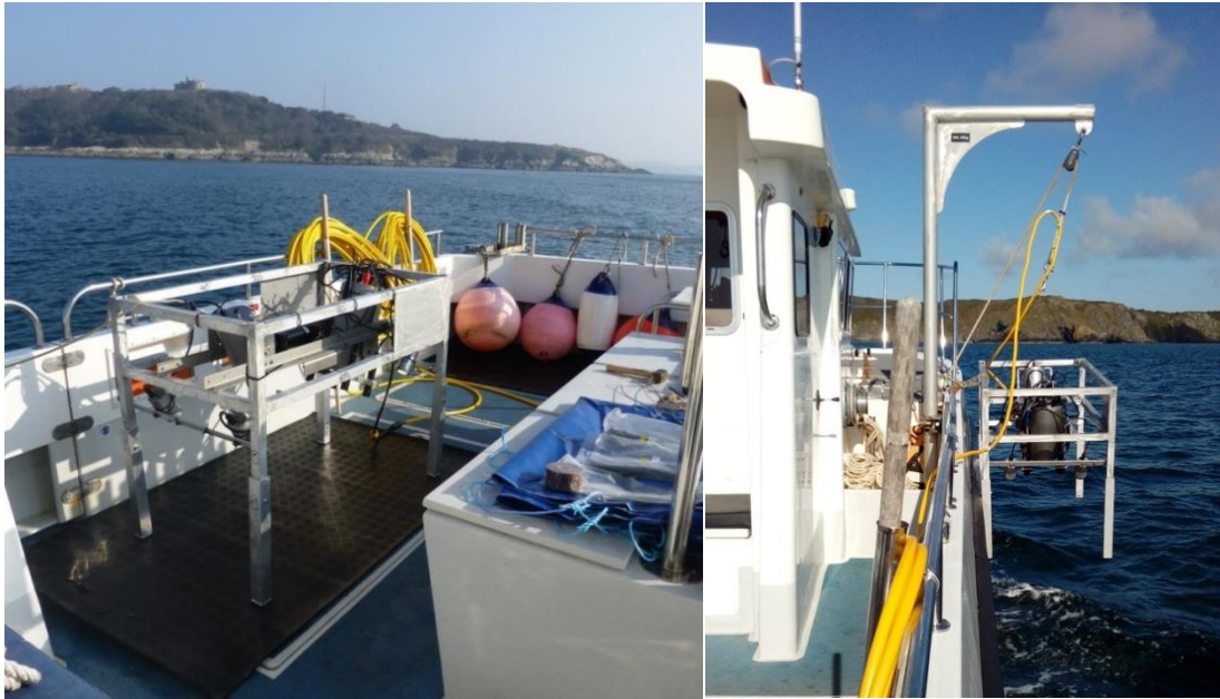
Figure 3: SeaSpyder drop camera housed in a purpose built frame on the aft deck and in the deployment position onboard R/V Tiger Lily VI.
