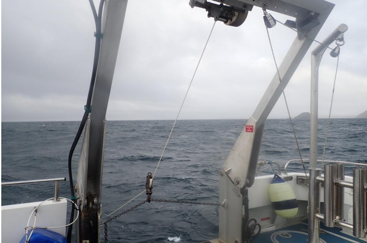
Figure 4: Lowered towing point on the A-Frame of R/V Tiger Lily with Dyneema towing cable running out to the N-Virodredge.
