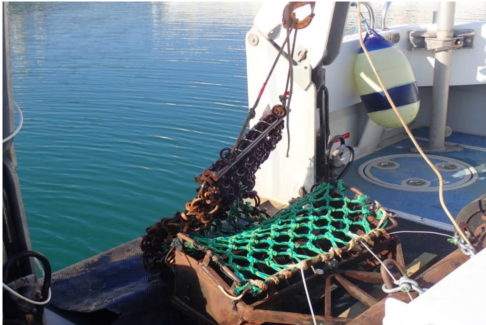
Figure 7: Slave hauler being used to raise the end of the dredge bag and empty the contents onto the deck of Tiger Lily
