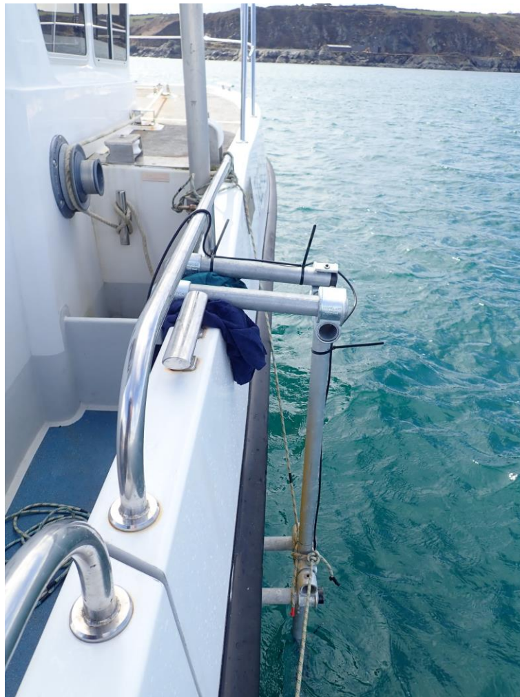
Figure 2: Mount setup on board R/V Tiger Lily for local beacon
