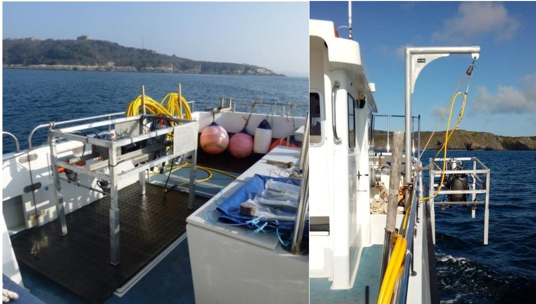
Figure 7: SeaSpyder drop camera housed in a purpose built frame on the aft deck and in the deployment position onboard R/V Tiger Lily VI.
