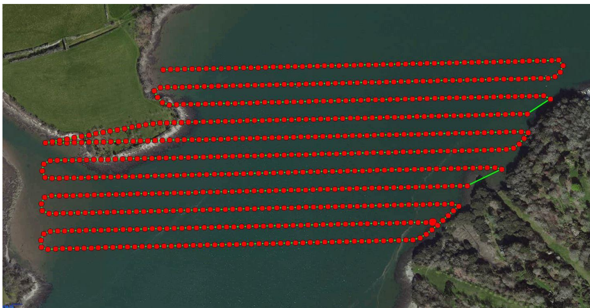
Figure 4: The pre-determined flight path showing individual camera locations for the broad scale flight by Vertical Horizons Media on 19 th September 2016
