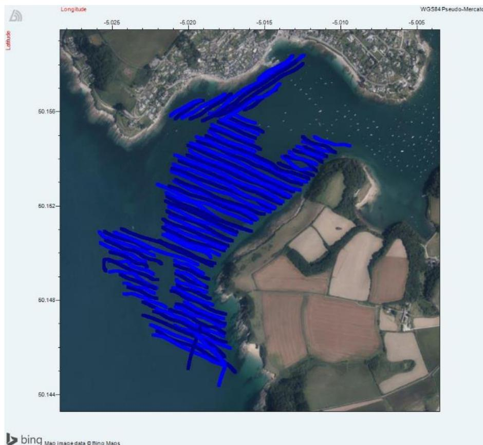
Figure 4: Acoustic survey lines completed at St.Mawes using an MX Echosounder by Cornwall IFCA 2021
