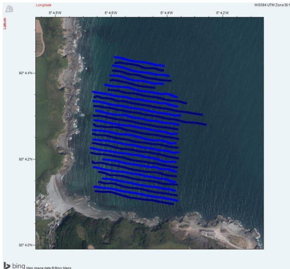
Figure 9: Acoustic survey lines completed at Porthallow using an MX Echosounder by Cornwall IFCA 2021
