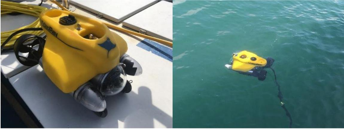
Annex Figure D: VideoRay Pro 4 Remotely Operated Vehicle deployed from R/V Tiger Lily VI
