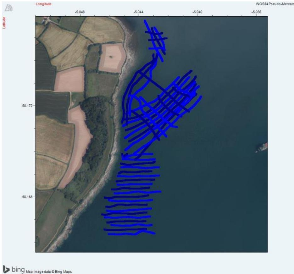
Figure 1: Acoustic survey lines completed at Penarrow Point using an MX Echosounder by Cornwall IFCA 2021
