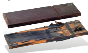
Opaque coated acetylated (top) and unacetylated Scots pine after 5 1/2 years outdoor test.
