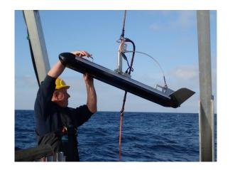
(L)map showing the planned side-scan sonar survey area and (R) deploying the side scan sonar from the Tiger Lily
