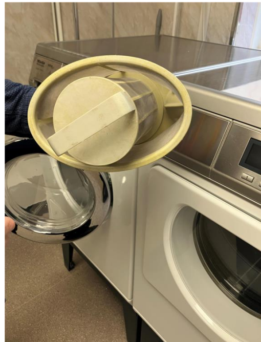
Filter seen to be clean and free from lint
