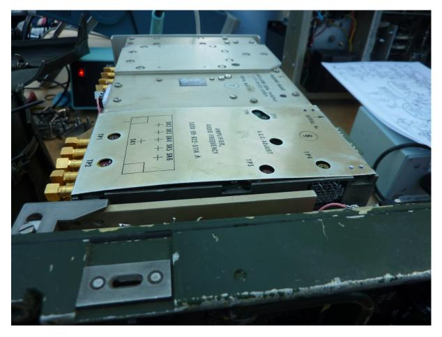
Remove the unit 6 cover, which is just clipped in place:
