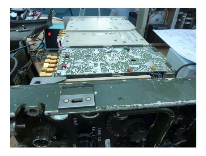
Desolder these joints only which carry AF (This is just for ease of manipulating the board). 321 joints are unusual in that you heat them up and with screwdriver at the same time, slide them back to disengage the joint, so freeing the module
