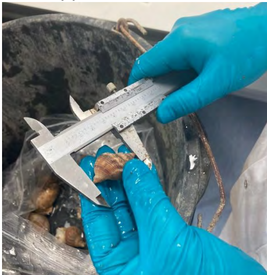
Officers measuring the total shell length of whelk samples using Vernier callipers.
