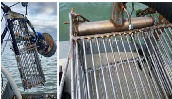
Figure 1. An example of the pump-scoop dredge used within the Poole Harbour Dredge Permit
