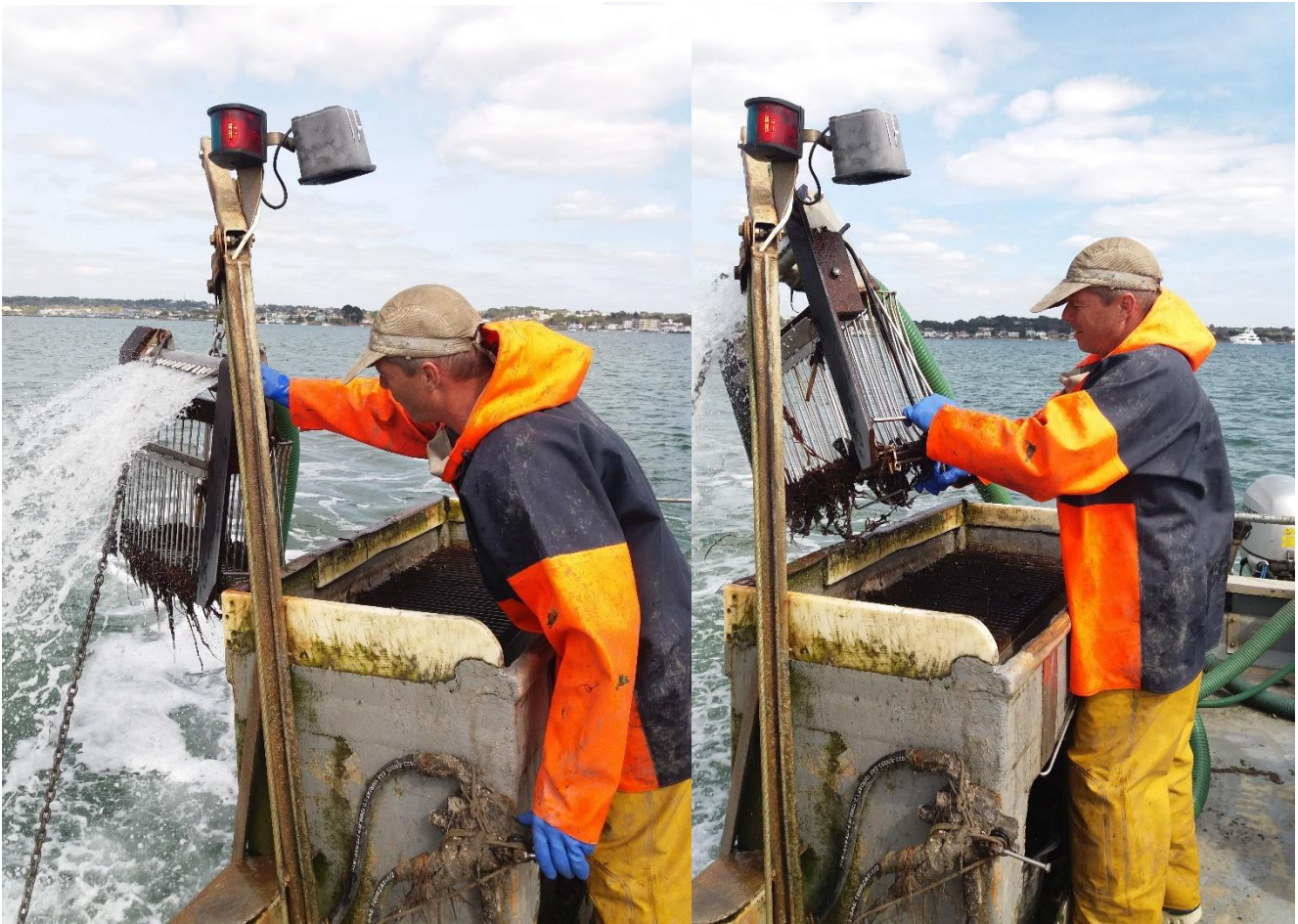
Figure 6. Typical pump-scoop dredge set up with basket dredge, water jets, davit arm and sorting riddle.
