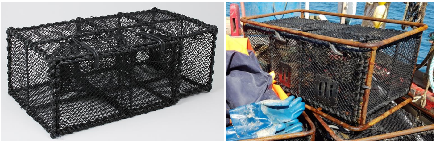
Figure 1. Fish trap used to catch wrasse (left) and fish trap fitted with metal frame and escape gaps (right).
