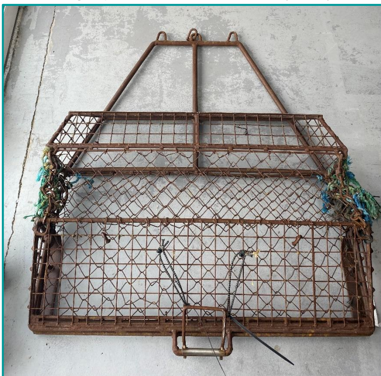
Figure 2: The Ladder Dredge.
