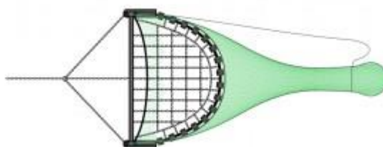
Figure 3. 'Chain mat gear' beam trawl.
