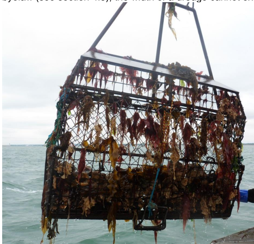
Figure 5. Ladder style oyster dredge similar to those used within the Solent oyster fishery.
