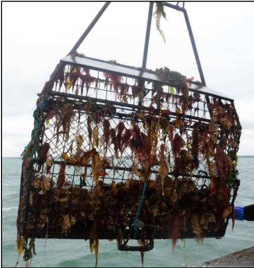
Figure 6. Ladder style oyster dredge similar to those used within the Solent oyster fishery.
