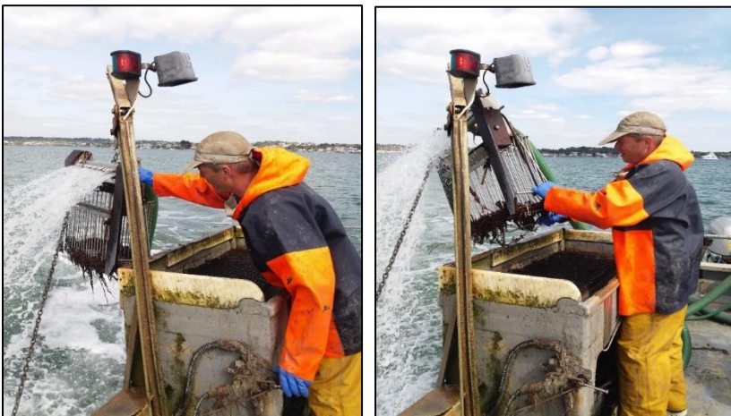
Figure 1. Typical pump-scoop dredge set up with basket dredge, water jets, davit arm and sorting riddle.
