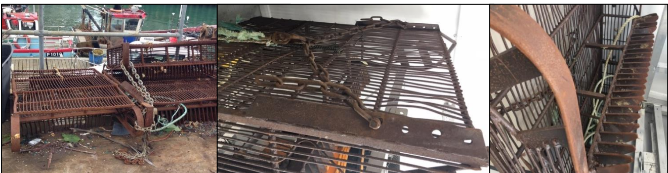
Figure 2. Box dredge used in the Solent clam fishery. Tow attachments. Dredge ski and teeth.
