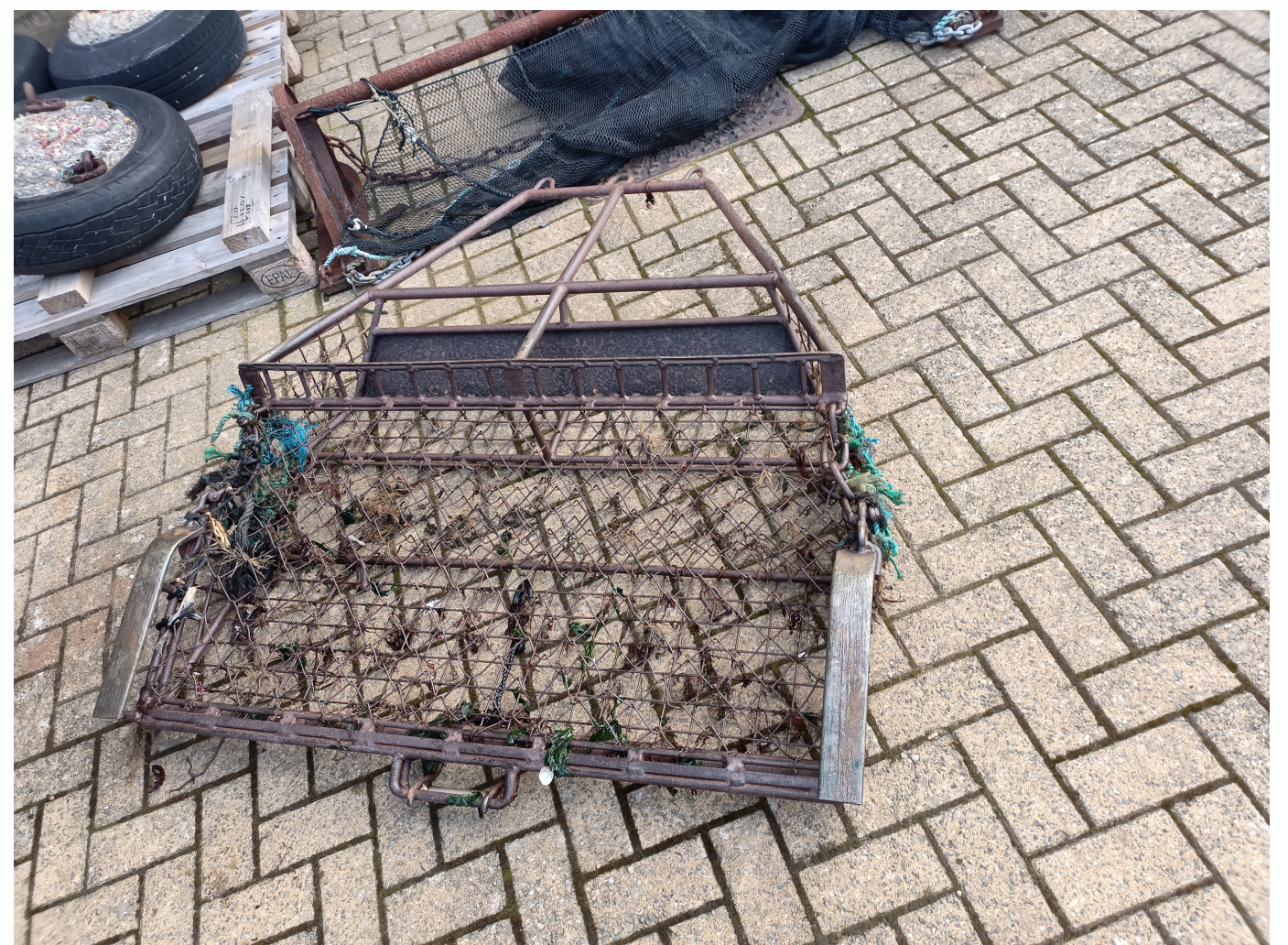
Figure 2 - The ladder dredge used for the Survey
