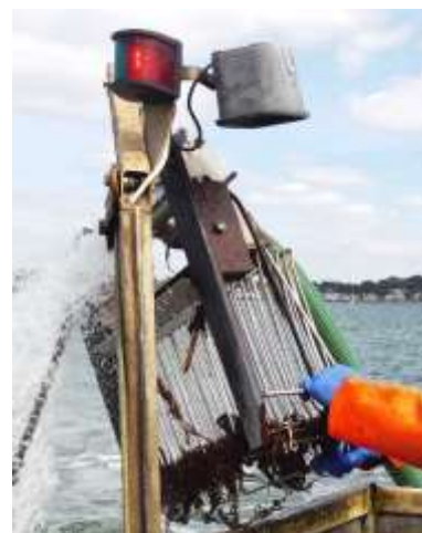
Figure 1. Photo of the trailed pump-scoop dredge used for bivalve sampling.
