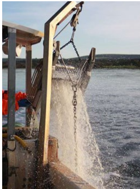
Figure 1. An example of the pump-scoop dredge which is used within the modern-day Poole Harbour Dredge Fishery to fish for clam and cockle species.
