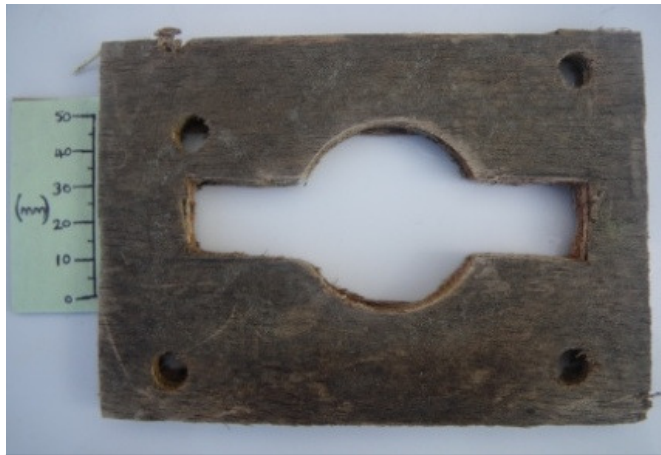
Figure 3.11. Hybrid escape gap design. With 20mm height of rectangle, and 48mm diameter circle.
