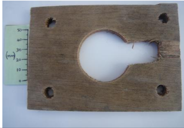
Figure 3.13. Half Hybrid escape gap. The design is similar to the hybrid escape gap, as 48mm circle is used, but only one side of the circle has the 20mm rectangle shape.
