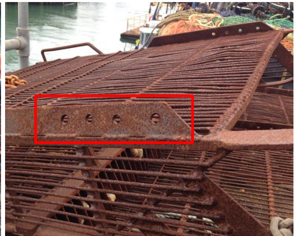
Figure 2. Box dredge tow riddle (highlighted in the red box). Two tow riddles are present on the front of the top of the riddle, one of each side. A rope attaches to the dredge through the holes in the tow riddle.
