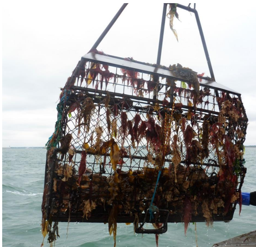
Figure 1. Ladder style oyster dredge similar to those used within the Solent oyster fishery.
