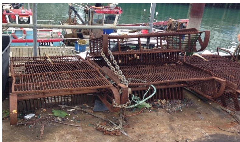
Figure 1. Box dredge used in the Solent clam fishery.
