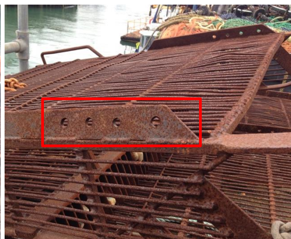
Figure 2. Box dredge tow riddle (highlighted in the red box). Two tow riddles are present on the front of the top of the riddle, one of each side. A rope attaches to the dredge through the holes in the tow riddle.
