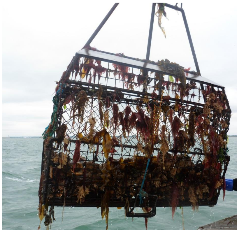
Figure 1. Ladder style oyster dredge similar to those used within the Solent oyster fishery. One or two dredges are deployed side by side, depending on the size of the boat, from the stern. The dredge is typically deployed using a mechanized winch to lower the gear to the sea bed and lift it back onto the vessel. The dredge is attached to the vessel using a metal wire and is towed along the seabed in straight lines in the direction of the boat. Once back on deck, the dredge is emptied onto sorting table where the catch is sorted and sized.
