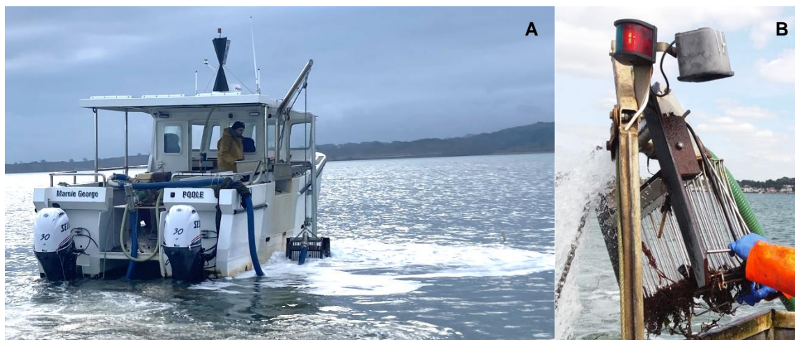
Figure 1: a) a permitted vessel in the Poole Harbour dredge fishery operating a pump-scoop dredge, b) the pump-scoop dredge
