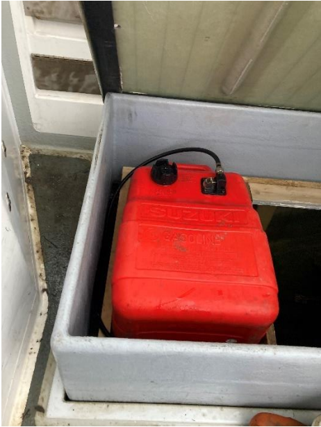
Figure 9: Developments to fueling mechanisms in the Poole Harbour dredge fishery through the use of in-board pumps which allows the fuel source to be contained within the vessel making the re-fueling process safer and improving the ability to contain any accidental spills
