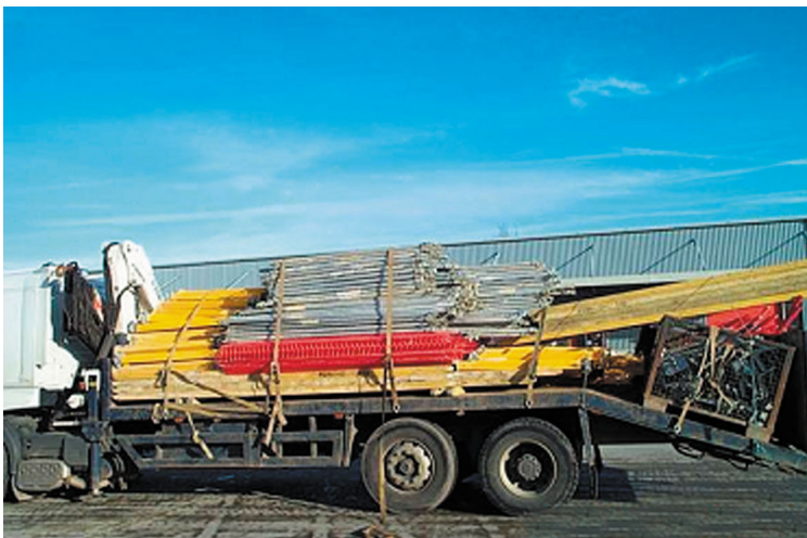
Figure 8. Vehicle unsafe to unload
