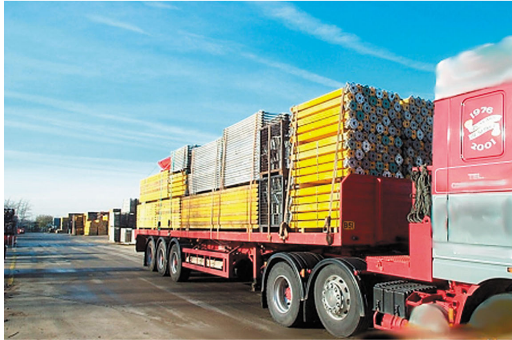
Figure 6. Example of a securely banded, spaced and strapped safe load
