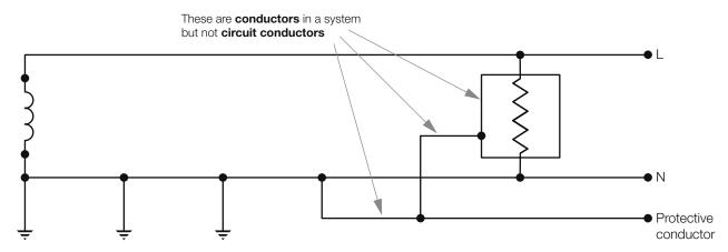
The combined neutral/earth conductor serves as both a neutral and a protective conductor and is therefore a **circuit conductor** as well as a **conductor in a system**
