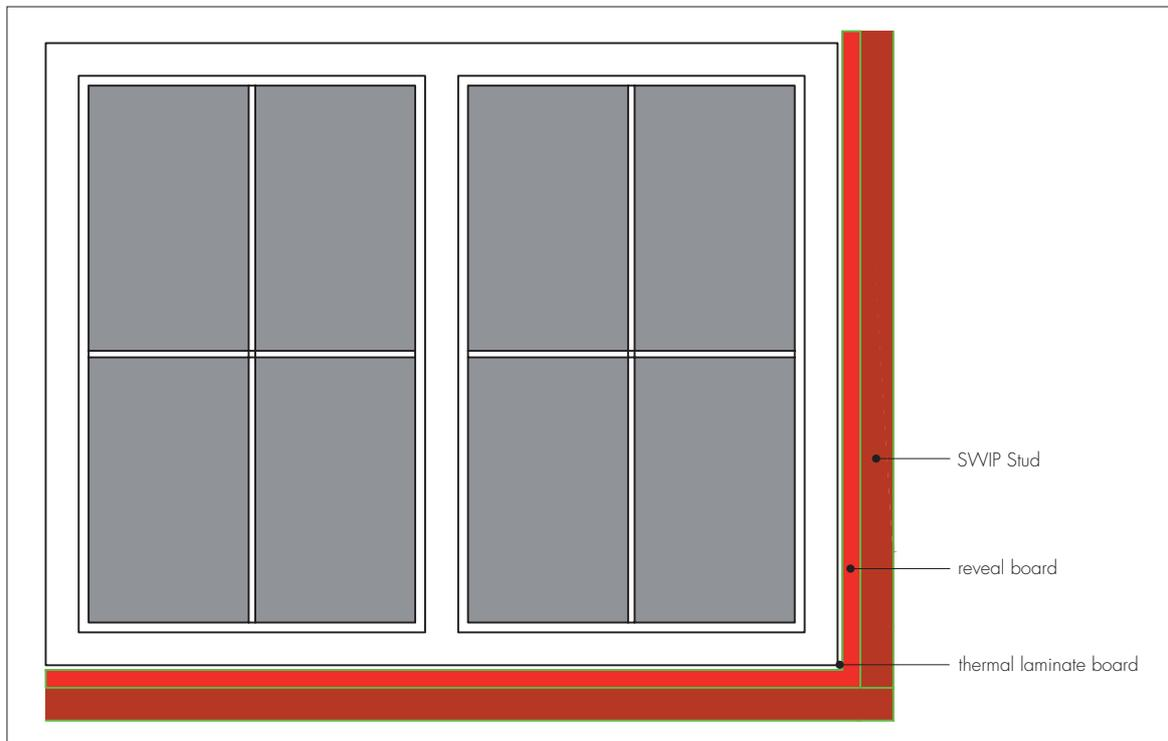
15.4 When setting out SWIP Studs adjacent to openings in relation to plasterboard dimensions, allowance must be made for the fact that the plasterboard needs to extend beyond the centre line of the jamb SWIP Stud to cover the thermal laminate board. For example, the dimension between the centre lines of the jamb SWIP Stud and the next SWIP Stud needs to be 600 mm, less the thermal laminate thickness (including adhesive dabs), less 25 mm (half the SWIP Stud width) (see Figure 6).
