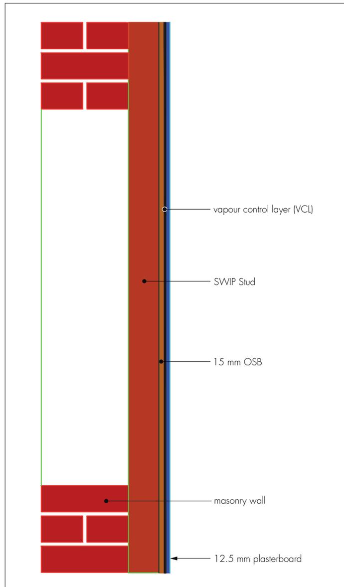
15.3 Openings are lined with a proprietary thermal laminate board (the Certificate holder can advise on suitable materials) and fixed using adhesive or plaster dabs, and additionally secured with localised mechanical fixings. The edge of the thermal laminate board should finish flush with the face of the SWIP Studs (see Figure 5).
