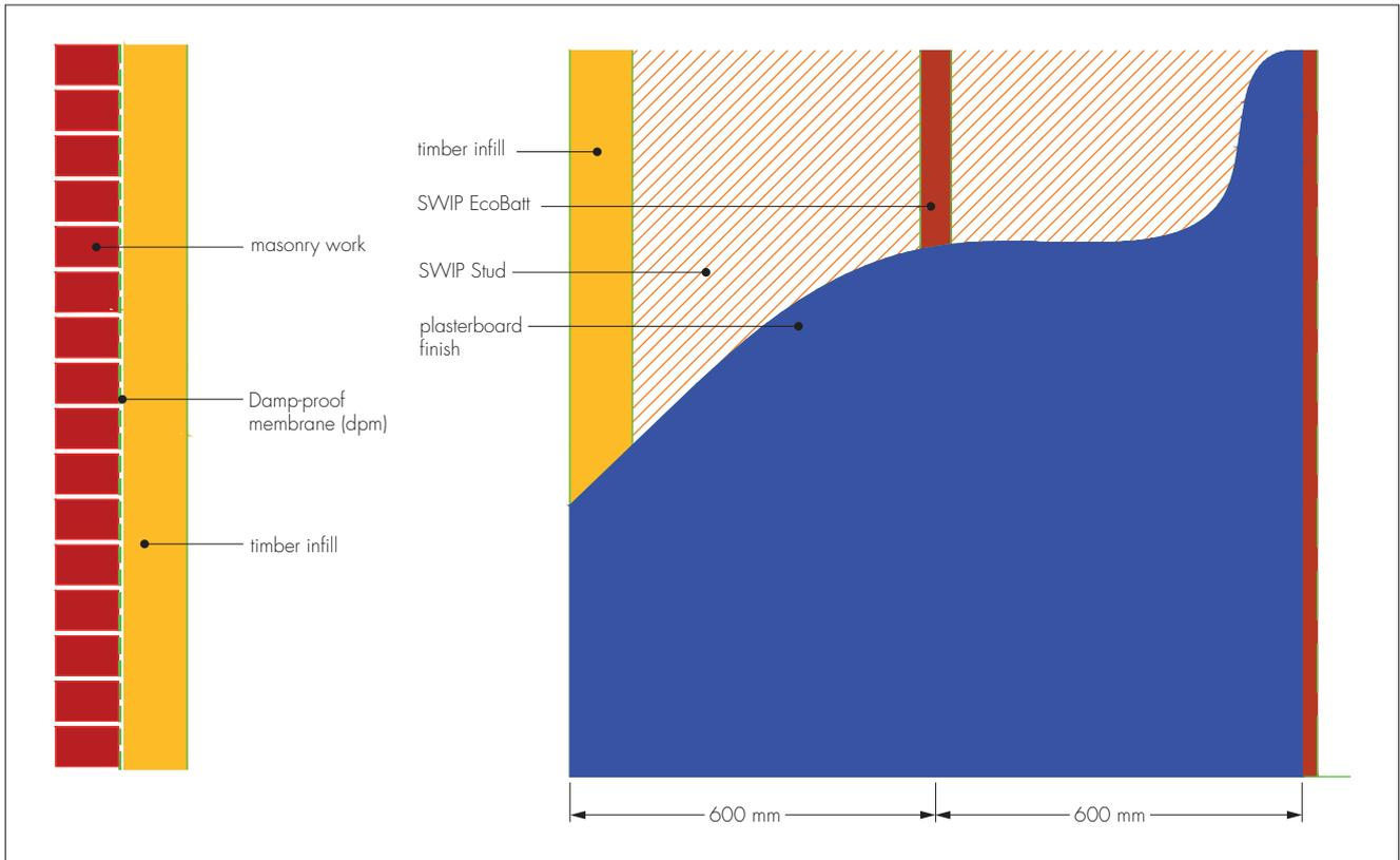
15.6 SWIP Studs are fixed to the face of the jambs and lined flush with the timber infill piece to form a continuous insulated lining around the opening. Plasterboard is cut back accordingly (see Figure 8).
