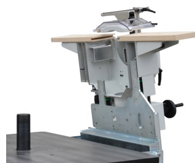
Esclusione cuffia toupie tramite supporto ribaltabile (opt) Revolving support To exclude the spindle hood (opt)
