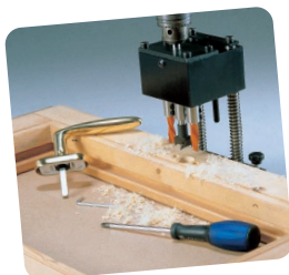
DRILLING FOR CREMONE BOLTS
