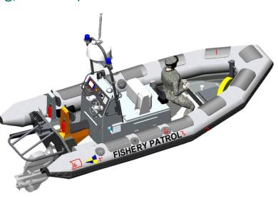
Stowed aboard FPV Watchful on her stern ramp, Osprey has been constructed to the highest standards, offering outstanding strength, stability, and seaworthiness. With a carrying capacity of up to four persons, her large inflatable tubes provide substantial reserve buoyancy and superior protection when operating alongside fishing vessels at sea.
