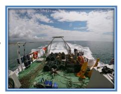
Deck plates can be installed where the Delta 1 RIB is situated to the stern of the ship. This allows for more working space during survey operations. The vessel has a large hydraulic deck winch and pot hauler, both of which can be utilised by the vessels crew to deploy a whole host of survey gear including beam trawls, towed video sleds, sidescan sonar and grab samplers.
