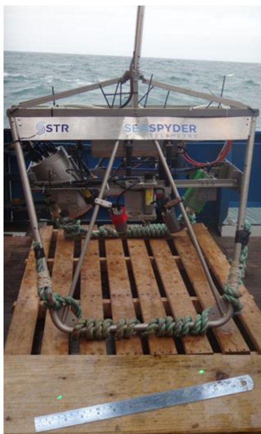
Figure 5. Drop Camera video and still imaging system.
